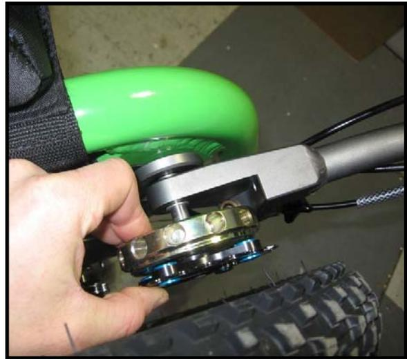
**For the left side (as sitting on the Trike) the Engagement Ring should turn the sprocket forwards when orientated as pictured.**
