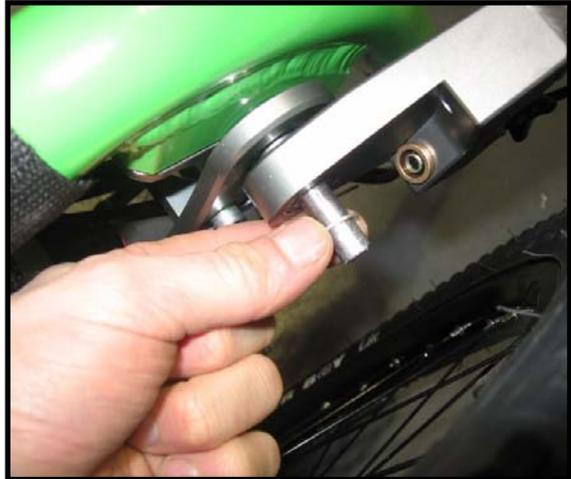
2. Slide Drive unit onto pivot pin – make sure it is the correct drive unit for that side of the trike. Check this by rotating the gold engagement ring (with holes in).
