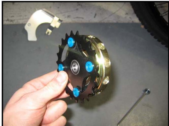
5. Unbolt Chain Ring, holding sprocket securely with Chain whip
