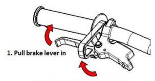
2. Rotate parking brake upwards to lock brake lever ON
