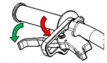
Rotate parking brake downwards – brake lever will spring outwards to release the brake
