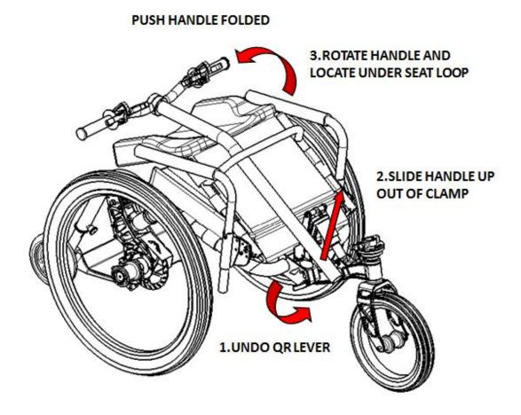
To refit the handle, slide it out from the seat back and slot in into the Clamp at the desired height. Ensure the handle is straight before tightening the Quick Release (QR) lever. (See instructions below for QR details)
