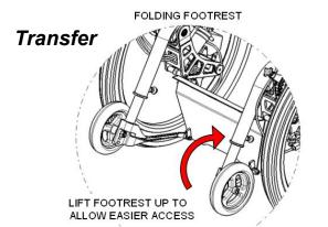
Do not stand on footrest during transfer. Lift the footplate up so it is out of the way, then fold down once seated
