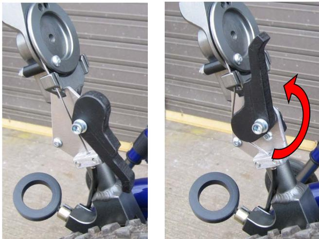
Please note: this parking brake is a new setup which allows the user to lock the brake and fold the drive lever down for easier access.
