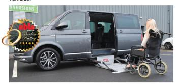
The Transporter can be configured for rear or side entrance, for drive from wheelchair or upfront passenger purposes (with flattened floor) as well as internal transfer - and is tested for wheelchairs up to 200kg. They also feature inboard or under floor lift options.
